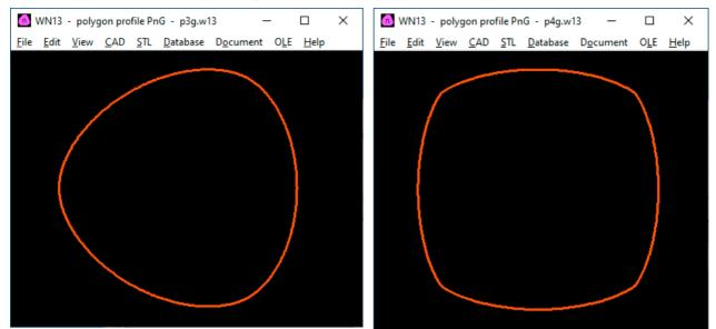
of teeth (P2G, P4G, P5G, P6G). WN13 thus replaces WN6, the calculation of dimensions and profile curve are identical. Surface pressure and minimum wall thickness are not calculated in accordance with DIN 32711, but in accordance with DIN 6892 (surface pressure parallel key connection) and DIN 7190 (minimum wall thickness of interference fit). Files from WN6 can be imported.
