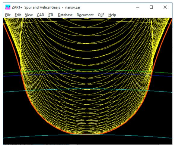
Dark blue: tooth root form diameter dFf Green: usable base circle diameter dNf (through counter gear) Light blue: base circle diameter db and tooth root diameter df
