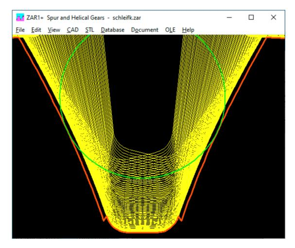
Once again a customer sent a tooth profile picture with an edge from the transition from the involute to the tooth root fillet with the question of whether this was a bug in the software. A check of his calculation file showed that a machining allowance q was entered, but a normal reference profile (no protuberance profile) was used. Then there are grinding notches, and these can also be seen in the tooth profile picture.
