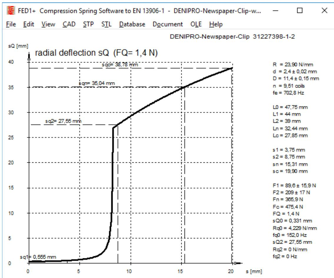
The transverse spring rate goes to 0 and remains 0 from  $s = s_k$ , when the spring buckles. The transverse force curves are interesting. If the spring does not buckle, the transverse spring rate may both increase or decrease, or both, depending on the distance to the buckling area.
