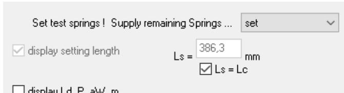
If "Ls = Lc" is checked under "Edit \ Production drawing" as setting length, then in new updates, only "Ls = Lc" will be output in the production drawing. If you want to output the block length in mm as before, remove the checkmark at "Ls = Lc".
