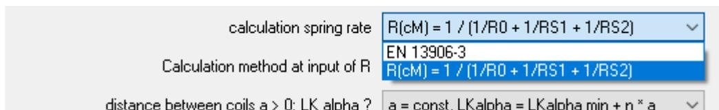
For legs on lever arm, the leg bending is calculated. If the suspension of the legs should also be taken into account when calculating the spring rate, this option can be set under "Edit \ Calculation method \ Spring rate calculation". A new warning "R leg > Ld / 10" appears if this option is not set and the lever arm of a supported leg is greater than 10% of the wire length.
