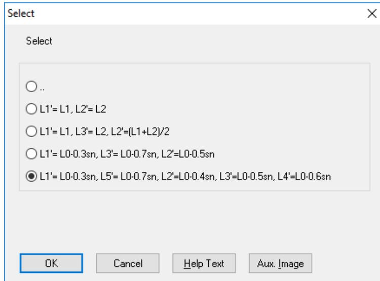
According to DIN 2096, the load-deflection curve between  $0.3 * sn$  and  $0.7 * sn$  is tested for hot-formed springs. Therefore,  $L1' = L0 - 0.3sn$ ,  $L3' = L0 - 0.7sn$  and  $L2' = L0 - 0.5sn$  were added as default for the input of the spring lengths, as well as for 5 measuring points  $Li' = L0 - 0.3, 0.4, 0.5, 0.6$  and  $0.7 * sn$ .
